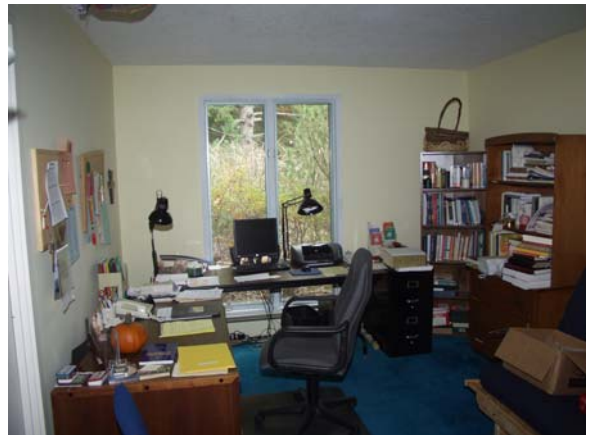
Task lamps compensating for lack of overhead lighting. In 1964, this space was appropriately served by table lamps, but these are not really effective for sustained use.
